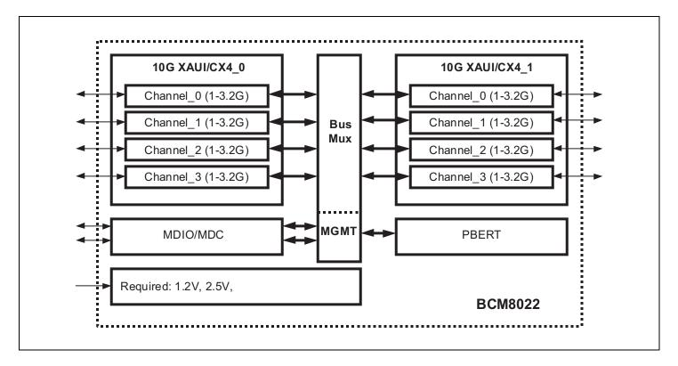
The BCM8022 device integrates four retimer channels leveraging Broadcom's high-performance mixed signal design experience along with advanced 0.13- $\mu$  CMOS process technology. Combine this with a robust architecture offering the highest degree of flexibility and the result is a highly programmable, lowest power retimer solution for network linecard and backplane applications.
